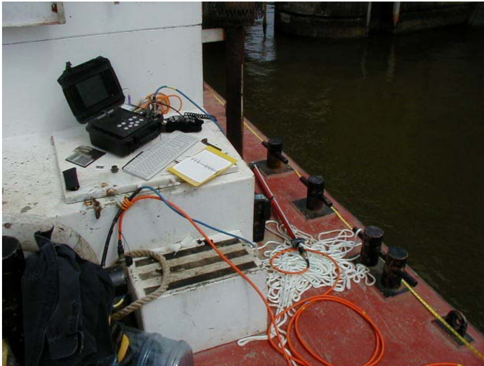
Figure 6.: GPR data collection system set up on the mini-tug.
