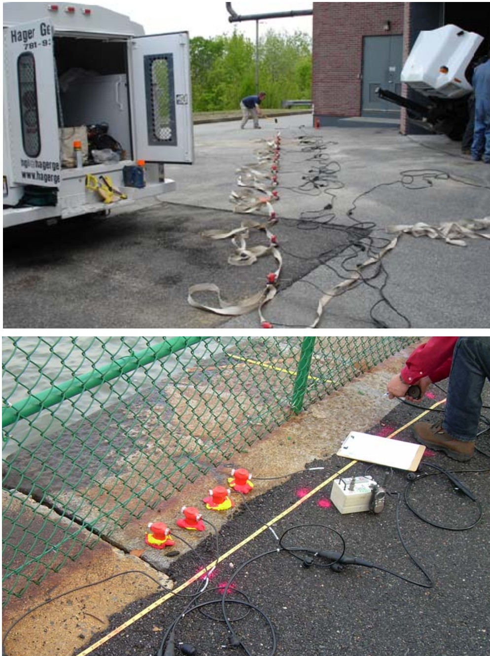
Figure 6: (top) MASW survey with geophones mounted on a land streamer, New Boston, NH; (bottom) impact echo survey with geophones coupled using modeling clay, NYC.
