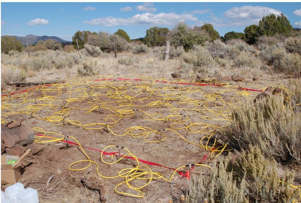
Figure 7: (top) ERT DAS-1 multiplexor; (bottom) 3D data acquisition survey geometry for a survey in Utah.
