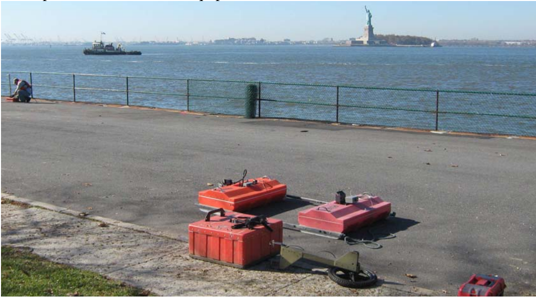
Figure 2: Mono-static 200-MHz and Bi-static 100-MHz antennas with survey wheel, NYC.
