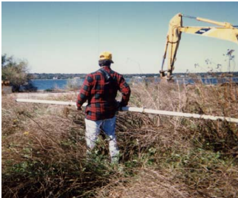
Figure 3: Mario Carnevale performing an EM-31 survey to map a reinforced concrete bunker tank on Gould Island near Newport, RI.
