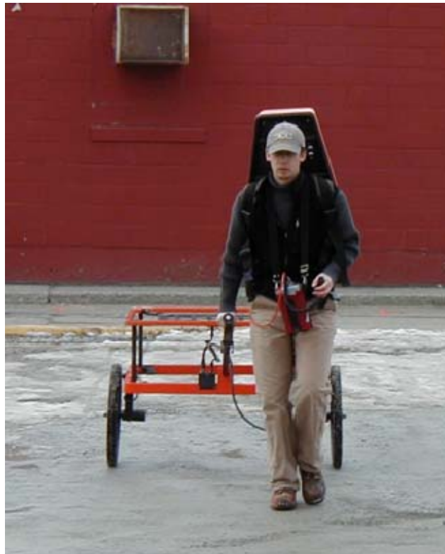
Figure 5: Alex Buller performing an EM-61 survey for USTs in an urban parking lot, St. Albans, VT.
