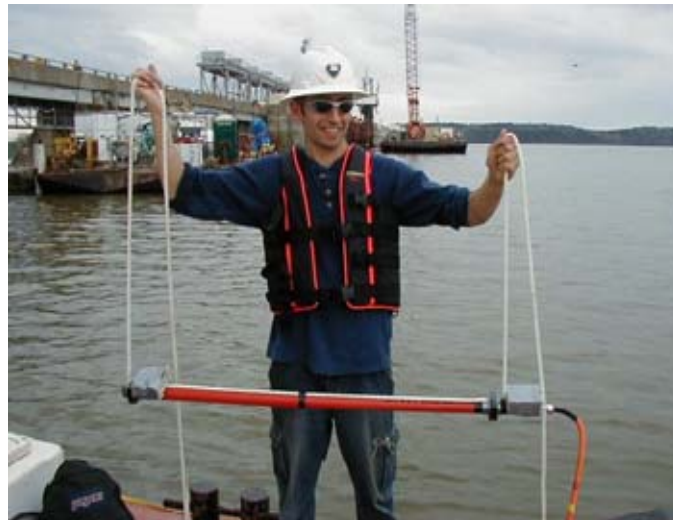
Figure 1: (top) GSSI MLF antenna configured to 20-MHz transmitting frequency for stratigraphic survey, ME; (bottom) 100-MHz Tubewave antenna for survey in 90-foot lake behind a dam, AL.
